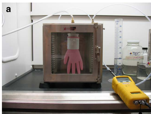
Figure 1. (a) Setup of permeation test. (b) Curve of permeation test. [Color figure can be viewed in the online issue, which is available at wileyonlinelibrary.com .]
